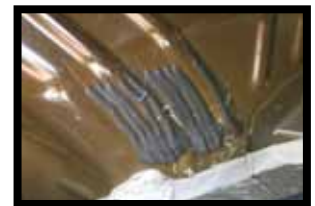
Photos from a 2011 Ford Mustang showing the sound deadener beads placed from the manufacturer in the trunk area.
