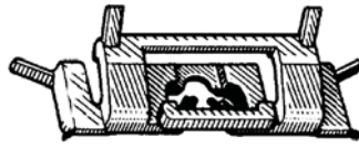
465140 HA01-50-609 Plastic Windshield Reveal Moulding Clip Mazda Truck '86 - UP Mercury Tracer '87 - UP Box Qty. 25
