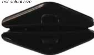
480513 20487630 Plastic Guide Front Door Window Guide GM Olds & Buick "C" Bodies '85 - UP Box Qty. 25
