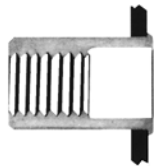
1. INSERT BLIND NUT INTO PREPARED HOLE.
