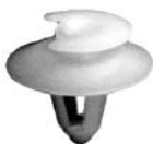
435417 124-990-04-92 Plastic Fender/Grille Drive-Type Rivet Hole: M7 Head Dia: 16mm Stem Length: 18mm Mercedes Benz C, CLK, CLS, E, M & R Class 2001 - UP Box Qty. 15
